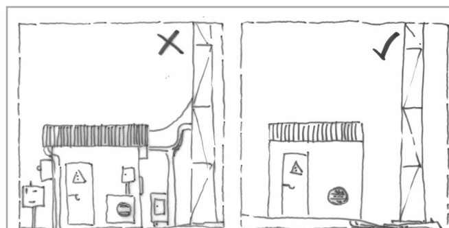
Accommodate mechanical equipment in container
